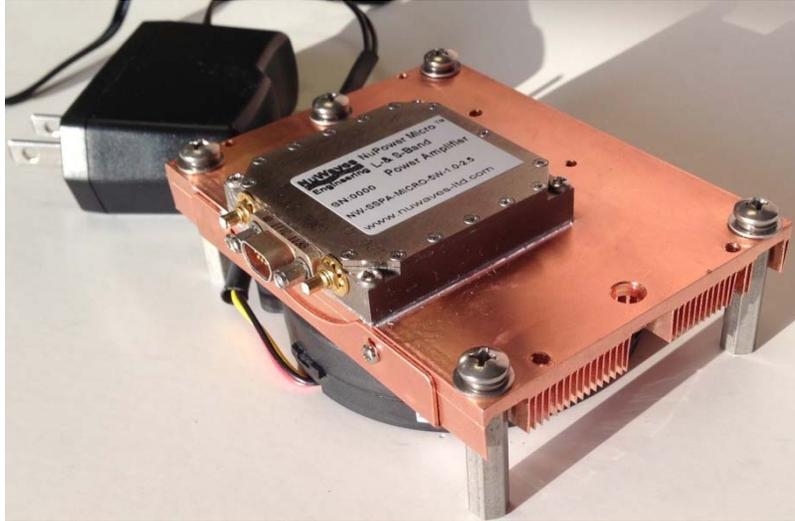
**Figure 3: The NuPower PA Kit offers “out-of-the-box” operation for the user. The fan-cooled heat sink with an AC/DC adapter is shown with an example PA (NuPower LS5MI01 not shown).**
