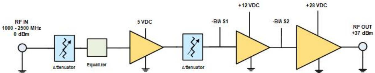
Figure 1: NuPower LS5MI01 Functional Diagram
