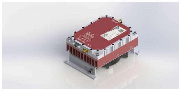
PA Module w/ Fan-Cooled Heatsink
