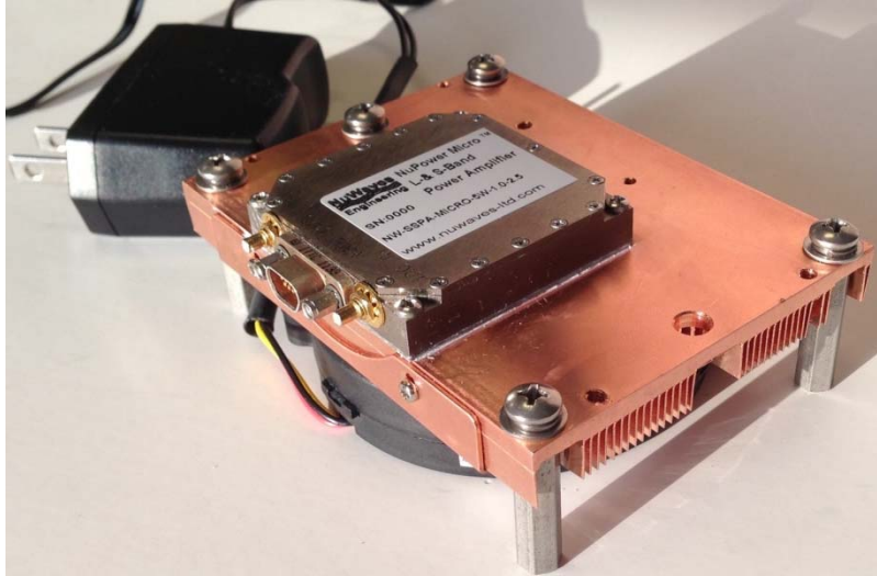
Figure 3: The NuPower PA Kit offers “out-of-the-box” operation for the user. The fan-cooled heat sink with an AC/DC adapter is shown with an example PA (NuPower 12A03A not shown).
