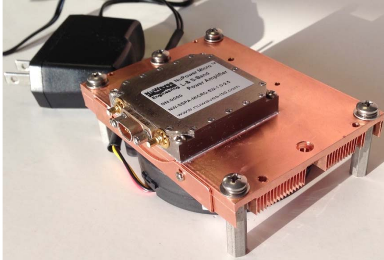
Figure 3: The NuPower PA Kit offers “out-of-the-box” operation for the user. The fan-cooled heatsink with an AC/DC adapter is shown with an example PA (NuPower 11C01A not shown).
