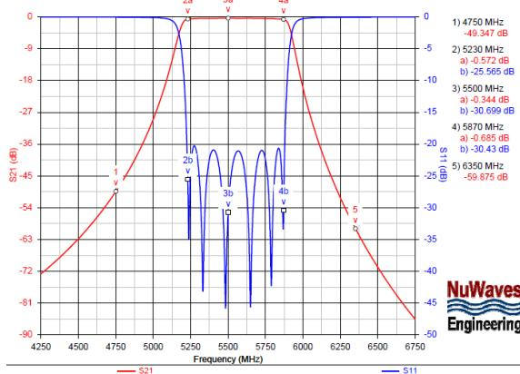
**Figure 2. Frequency Response of the C-Band Cavity Filter shown in Figure 1 (Bandpass Filter). Cavity Filters provide high ultimate rejection, with low passband insertion loss.**
