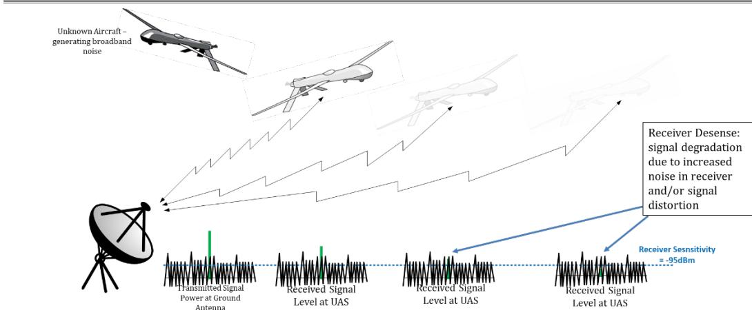
**Figure 4. A second UAS, broadcasting wideband RF noise significantly reduces the communications range between the Ground Station of the first UAS. Using a narrow bandpass filter at the UAS receiver will improve system performance, but some noise will still enter the receiver and reduce the range.**
