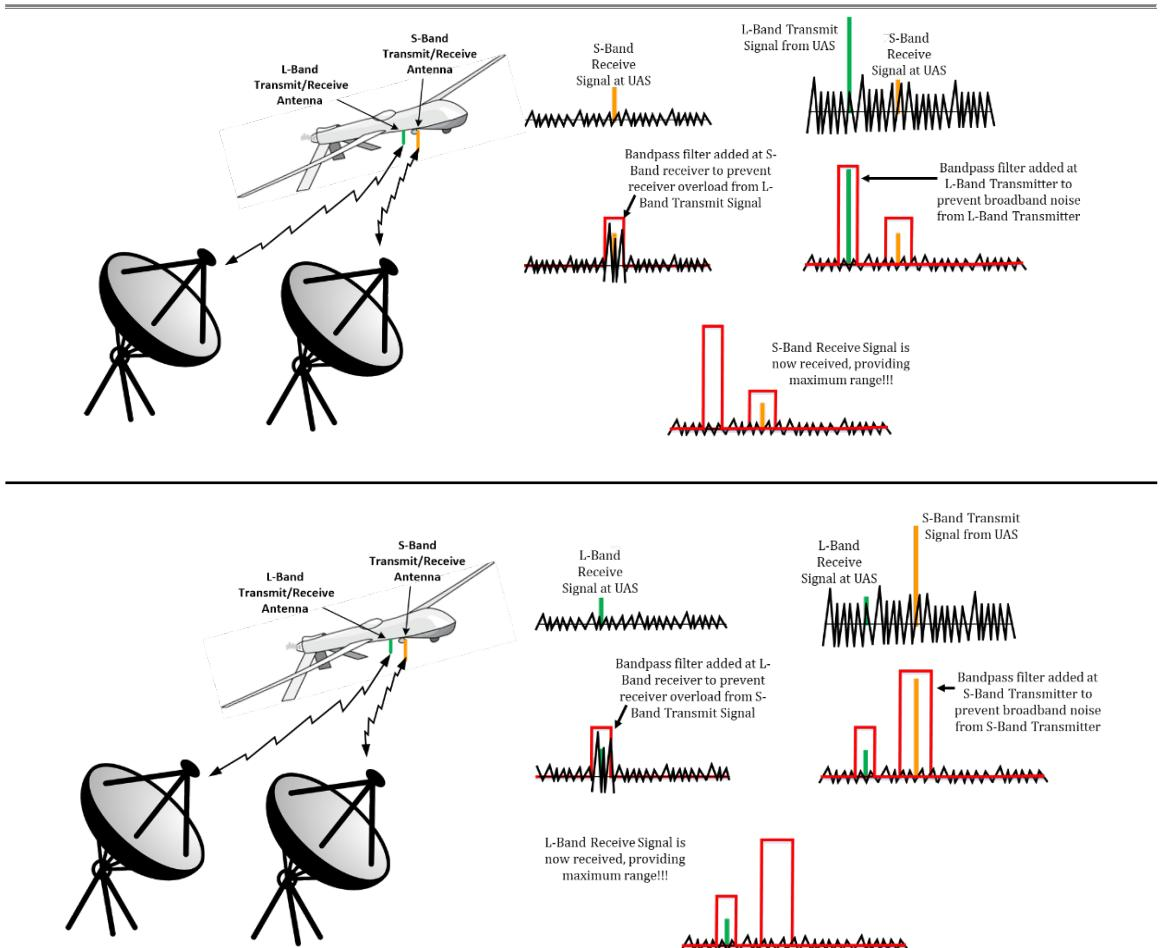
**Figure 8. The broadband noise created by the L-band and S-band transmitters in the UAS payload are reducing the receiver sensitivity of the S-band and L-band receivers, respectively. By installing bandpass filters at the output of each transmitter, the interference is mitigated.**
