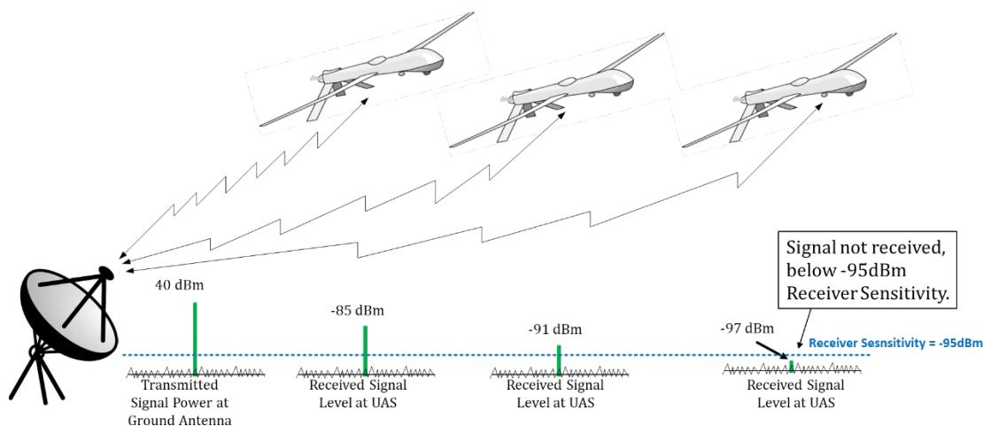
**Figure 3. The UAS is traveling in an ideal RF environment, and is able to travel the maximum distance from the Ground Station before the link is lost.**
