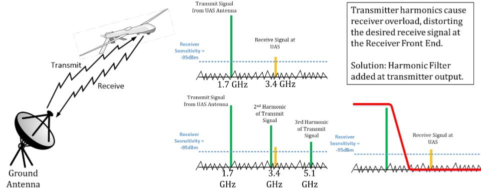
**Figure 7. An onboard transmitter and RF power amplifier creates harmonic radiation that prevents the reception of the desired signal. By installing a harmonic filter on the output of the power amplifier, the interference is mitigated.**
