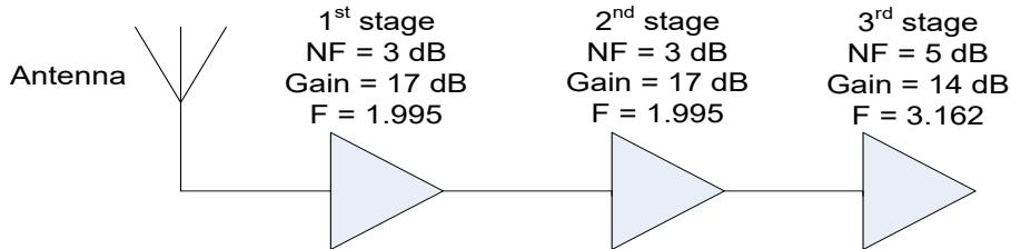
**Figure 2. The notional receiver used as an example in this application note has a first stage NF of 3 dB.**
