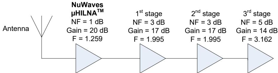
**Figure 3. The  $\mu$ HILNA™ is inserted between the antenna and the notional receiver, improving the NF of the system by approximately 2 dB.**
