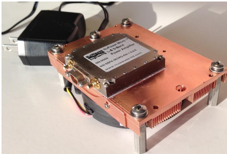
Figure 3: The NuPower PA Kit offers “out-of-the-box” operation for the user. The fan-cooled heatsink with an AC/DC adapter is shown with an example PA (NuPower 12B01A-D30 not shown).
