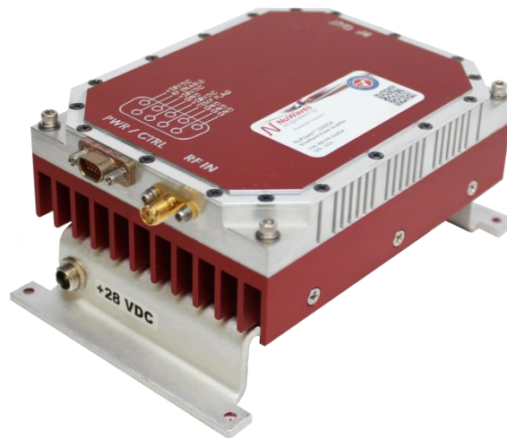
Figure 3: The NuPower PA Kit offers “out-of-the-box” operation for the user. The fan-cooled heatsink is shown with an example PA (NuPower Xtender SCISR-20-C01-S01 not shown).
