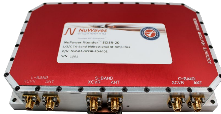
Figure 2. The NuPower Xtender SCISR-20 Tri-Band Bidirectional Amplifier capitalizes on the extreme power density and frequency flexibility offered by GaN to deliver 20 W Psat in L/S-bands and 10 W Psat in C-band. This tremendous capability comes in a small form factor at just 7.25" x 4.50" x 1.375", roughly the size of a typical novel.
