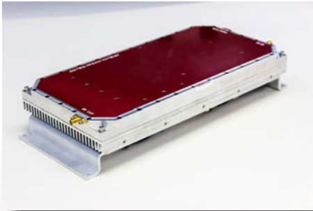
Integration of a high power RF amplifier for use in military platforms.
