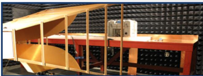
In-house Military Standard, DO-160 Standard, and system level testing for application specific and platform certification. NuWaves frequently designs and tests to MIL-STD documents and we quickly and cost effectively meet stringent system level qualification requirements. NuWaves has an in-house anechoic chamber, vibration/shock table, and temperature and humidity chambers to test a wide range of EMI/EMC and environmental conditions for military applications.
