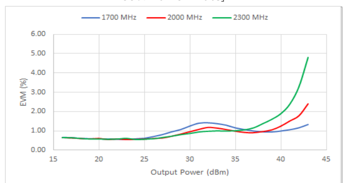
Error Vector Magnitude vs. Output Power [QPSK, 1Msps, 35% Roll Off Rate]
