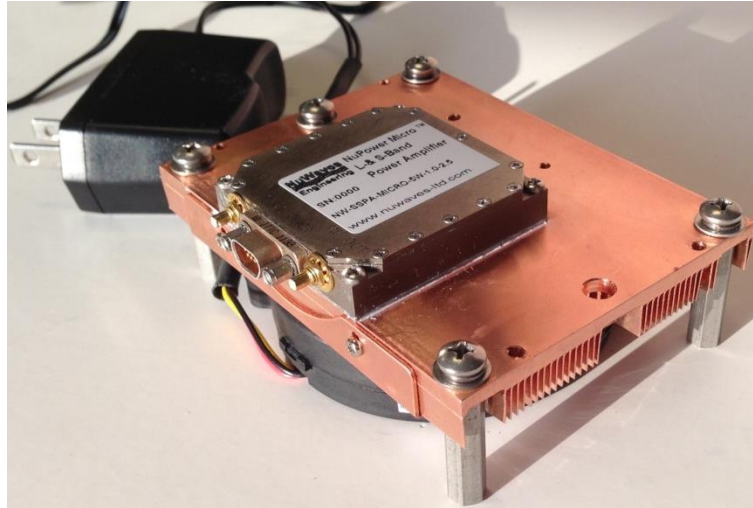
Figure 3: The NuPower PA Kit offers “out-of-the-box” operation for the user. The fan-cooled heatsink with an AC / DC adapter is shown with an example PA (NuPower ULS-25-C01-S01 not shown).
