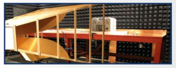
In-house Military Standard, DO-160 Standard, and system level testing for application specific and platform certification. NuWaves frequently designs and tests to MIL-STD documents and we quickly and cost effectively meet stringent system level qualification requirements. NuWaves has an inhouse anechoic chamber, vibration/shock table, and temperature and humidity chambers to test a wide range of EMI/EMC and environmental conditions for military applications.
