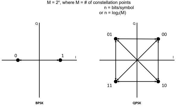
Figure 4. State diagrams for BPSK (left) and QPSK (right).
