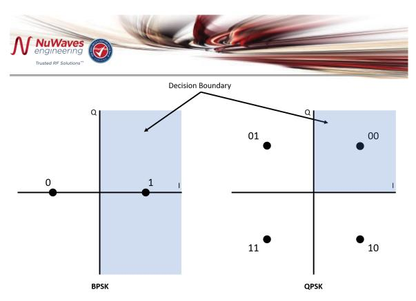
Figure 5. Decision boundaries for BPSK (left) and QPSK (right).
