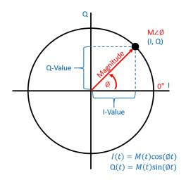
Figure 2. I/Q diagram superimposed on polar diagram.
