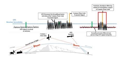
Figure 5. The transmitter on the UAS is transmitting RF noise in the GPS frequency band, causing the GPS receiver to lose GPS signals. By filtering the output of the transmitter, the interference to the GPS receiver is eliminated.
