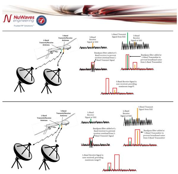
Figure 8. The broadband noise created by the L-band and S-band transmitters in the UAS payload are reducing the receiver sensitivity of the S-band and L-band receivers, respectively. By installing bandpass filters at the output of each transmitter, the interference is mitigated.
