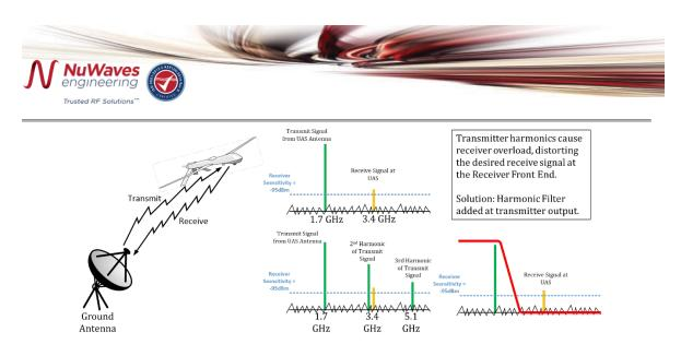
Figure 7. An onboard transmitter and RF power amplifier creates harmonic radiation that prevents the reception of the desired signal. By installing a harmonic filter on the output of the power amplifier, the interference is mitigated.
