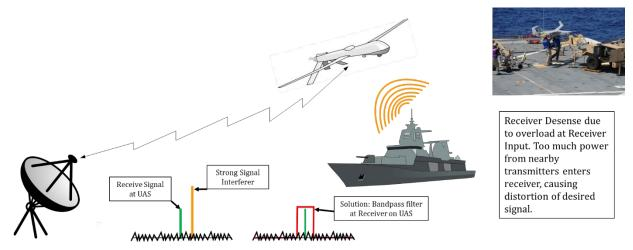
Figure 6. The presence of a strong signal transmitted from the ship overloads the UAS receiver, and the link to the Ground Station is lost. A bandpass filter on the input of the receiver filters out the interfering signal.
