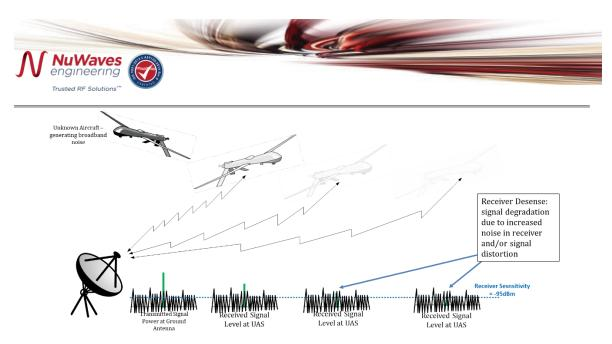
Figure 4. A second UAS, broadcasting wideband RF noise significantly reduces the communications range between the Ground Station of the first UAS. Using a narrow bandpass filter at the UAS receiver will improve system performance, but some noise will still enter the receiver and reduce the range.
