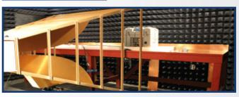
In-house Military Standard, DO-160 Standard, and system level testing for application specific and platform certification. NuWaves frequently designs and tests to MIL-STD documents and we quickly and cost effectively meet stringent system level qualification requirements. NuWaves has an inhouse anechoic chamber, vibration/shock table, and temperature and humidity chambers to test a wide range of EMI/EMC and environmental conditions for military applications.
