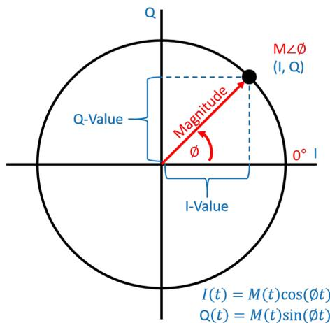
**Figure 2. I/Q diagram superimposed on polar diagram.**
