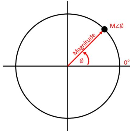
**Figure 1. Polar diagram representing amplitude (magnitude) and phase.**
