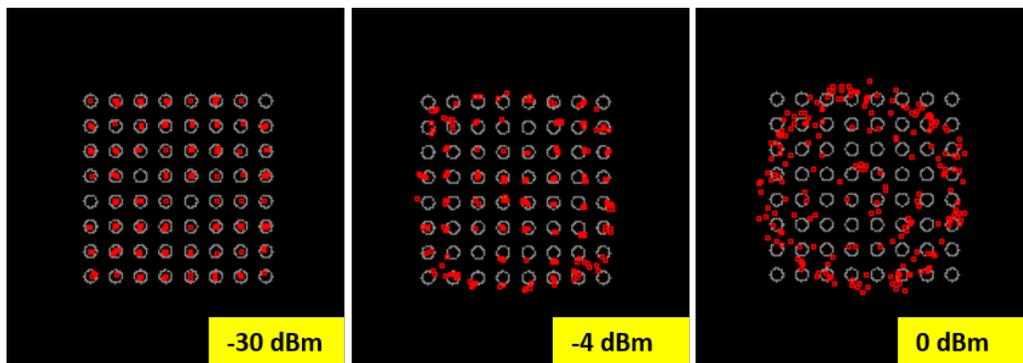
**Figure 7. Measured signal symbols (red dots) increasingly misaligned with ideal signal constellation points (white circles) due to greater signal distortion as input drive level increased from -30 dBm to 0 dBm.**
